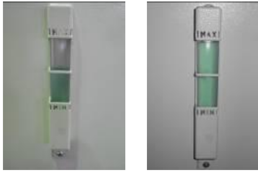
Picture 18 / 19 – Tank top up
