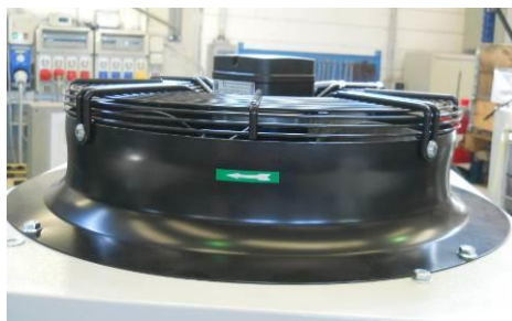
Picture 20 – Example of fan rotating direction
