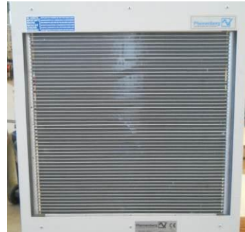
Picture 24 – Condenser external surface
