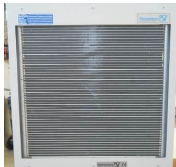
Figure 24 – Surfaces externes condenseur
