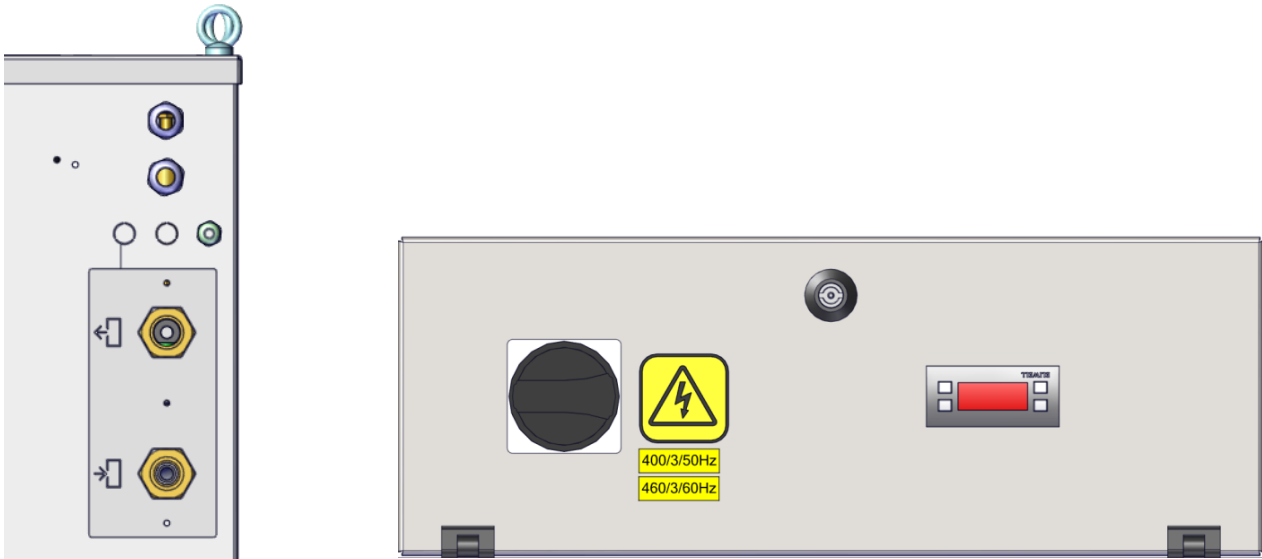
Picture 11b – Electrical connections with labels (3-Phases), the labels are on the Electrical Box.
