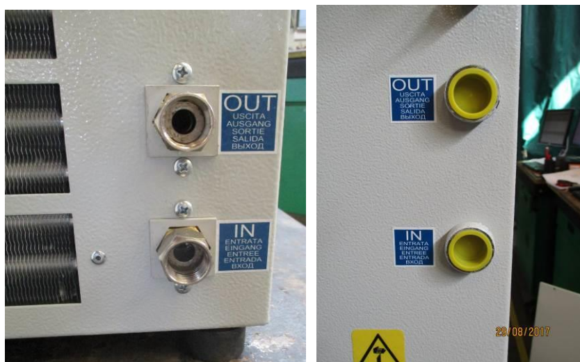
Figure 3 / 4 - Plaque de connexion hydraulique
