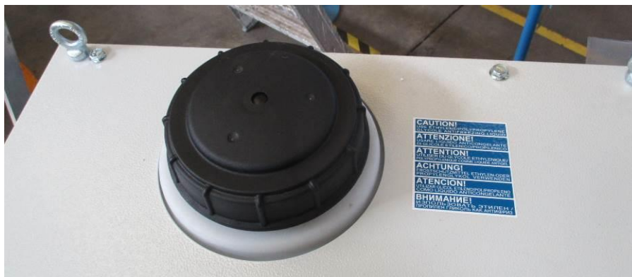
Picture 9 – Example of filling point
