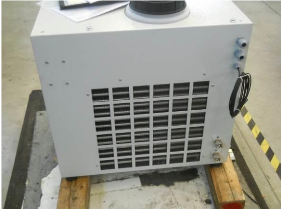
Picture 20 – Condenser external surface for CCE 6101 – 6201 – 6301
