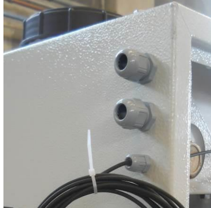
Picture 5 – Electric connection
