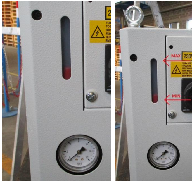
Picture 14 / 15 – tank top up
