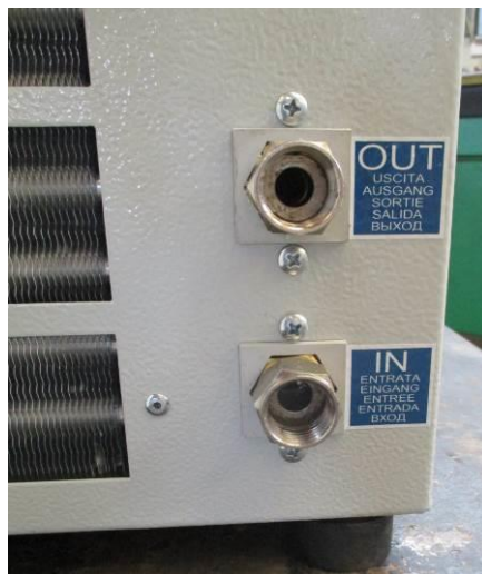
Picture 3 –Hydraulic connection plate
