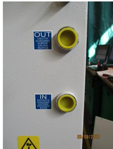
Picture 4 –Hydraulic connection plate
