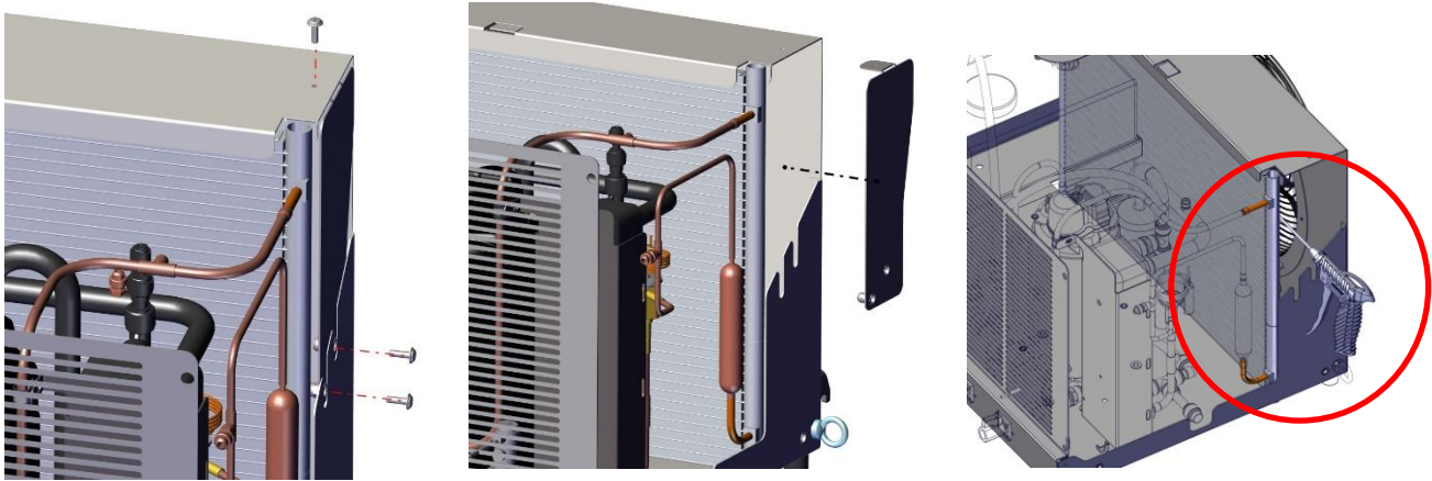
Picture 18 – Condenser cleaning
