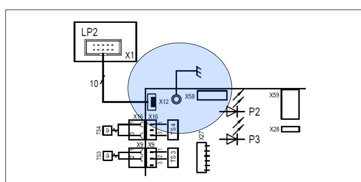
Figura 14: Interfaz Modbus RTU (X58)
